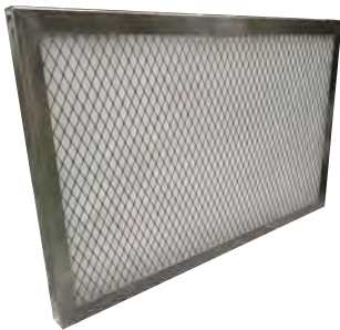
Unique SS Expanded Mesh for air filter and corrosion resistant applications FC SS304 Frame,SS304 Expanded Mesh, SS304 Z-Zag Rod Typical Nominal thickness" 0.5,1,2,4" Actual Thickness 12,21,45,95mm
