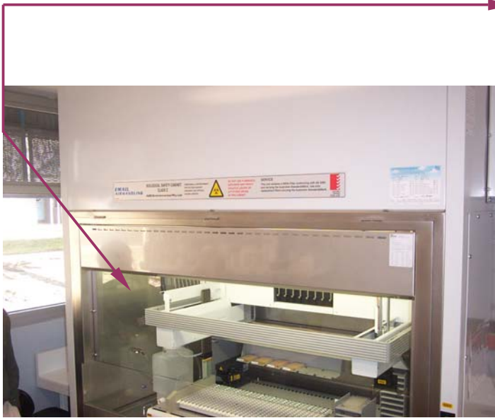
TECAN EVO 150 Robotic Sampler housed in our 1800mm Class II Cabinet.
