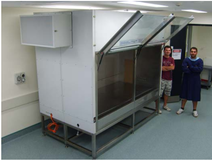
Purpose built Class II Biological Safety Cabinets to house Robotic Samplers
