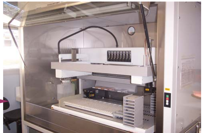
TECAN EVO 150 Robotic Sampler housed in our 1800mm Class II Cabinet.
